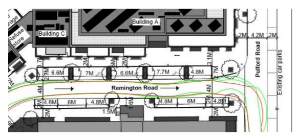
For access the refuse trucks will pass along Remington road, this presents a conflict as there is not the width for the truck to pass by the planned trees, there are 10 tree's along the route that a truck would pass through (green lines represent the swept path of the trucks body, red lines the swept path of the trucks, its particularly bad at the end of the road where there is a double row of trees planned. As refuse trucks are 4m high they won't pass under trees canopy but push through it.
